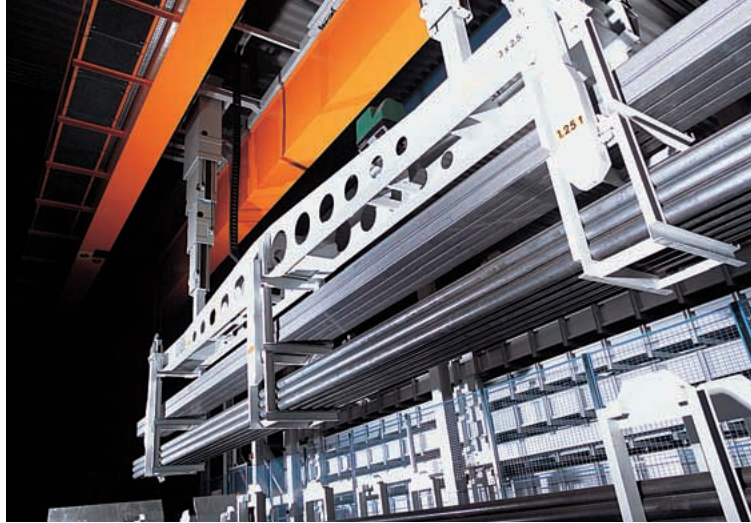
Fast transport: Multiple lift spreader beam with three adaptor pairs and telescopic guide while moving 2 storage layers.
