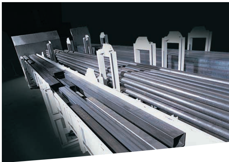
Flexible storage: Even remnants can be optimally stored by using stacking cradle cassettes.
