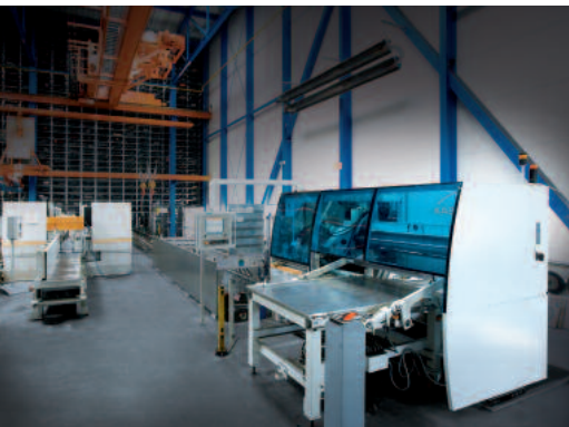
KASTO saws at a buffer station.
