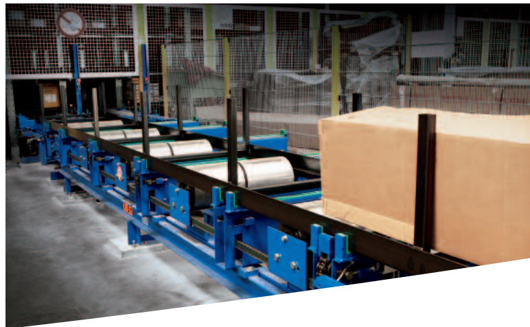
Station with integrated roller conveyor.
