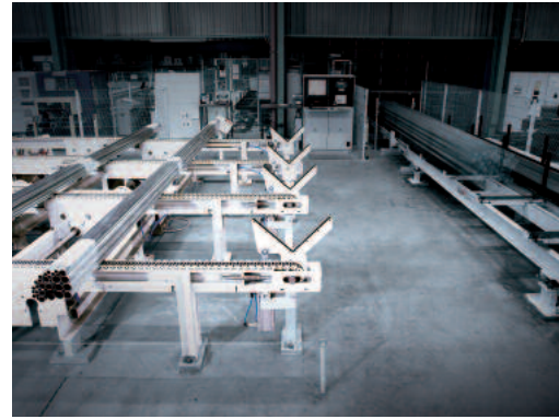
Vertical rotary station at front of storage system with ten logical locations.
