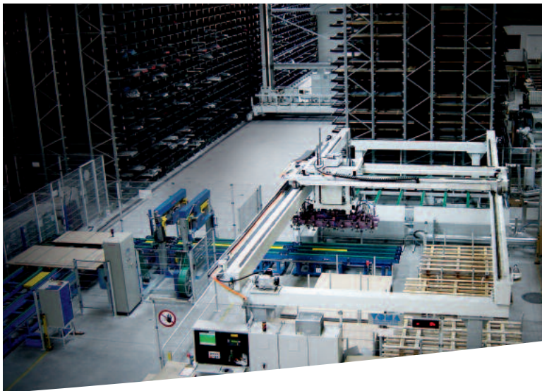
Honeycomb system for bar stock/sheets with fully automatic sheet commissioning system.
