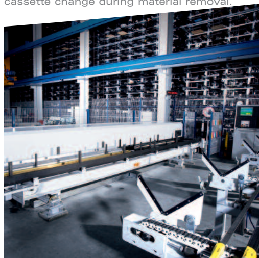
Rotary station at longitudinal side of storage system with protective cover for cassette change during material removal.
