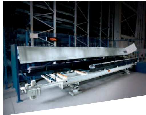
Storage system with lift unit and stop portal for easy storage of customer-own bar stock cradles via forklift.
