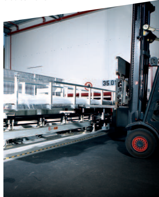
Storage system with lift unit and stop portal for easy storage of customer-own bar stock cradles via forklift.
