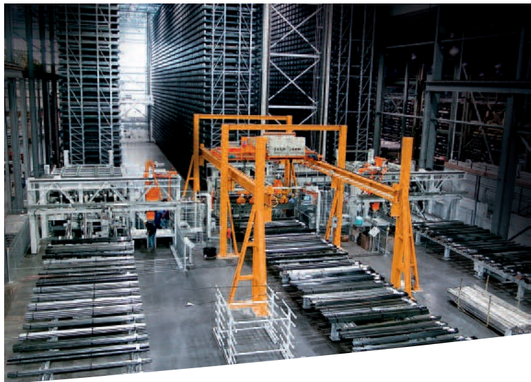
UNICOMPACT with three shelf blocks and two operating gantry cranes.
