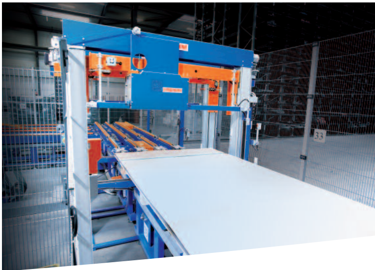
Fully automatic, integrated wrapping unit with conveyor system.
