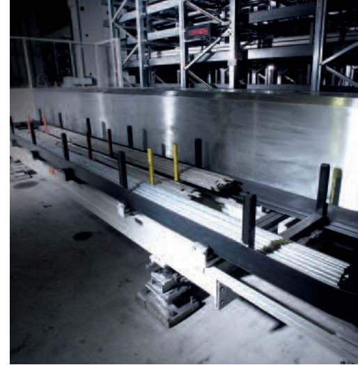
Cassette at rotary station with protective cover.
