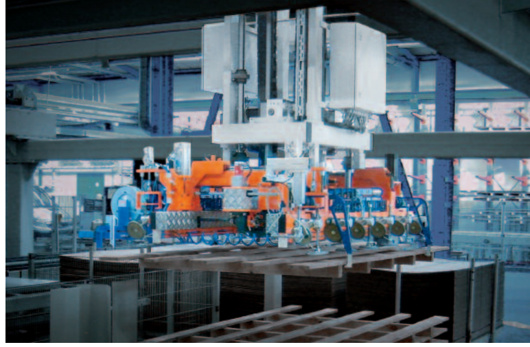
Fully automatic sheet metal manipulator.
