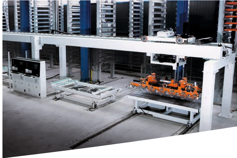
Automatic commissioning station with vacuum sheet lifter.
