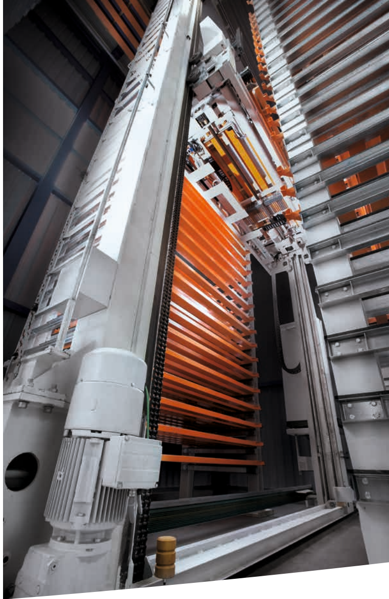
Operating gantry crane with proven chain hoist.
