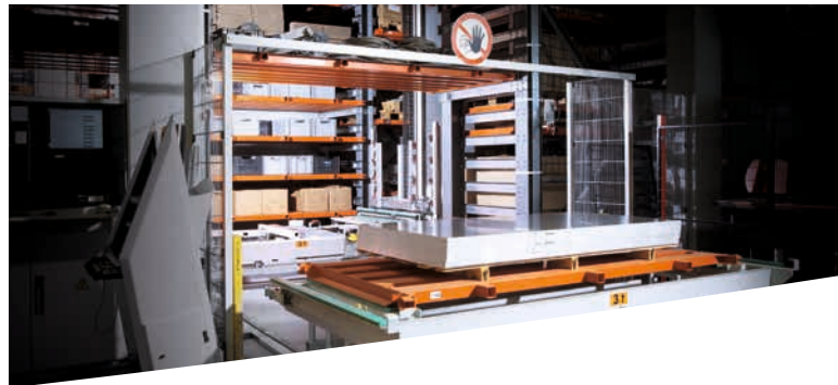
Storage and removal station designed for two different pallet sizes to universally store different products.
