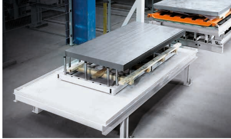
Unpacking table with movable frame and storing/removal station.
