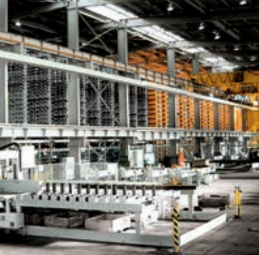
Sawing center with bandsaw and palletizing technology at a service center in Japan.
