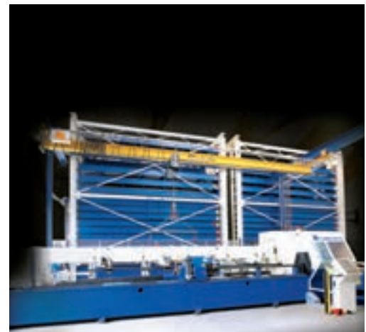
Double tower for tubes as a buffer stock for a tube laser processing machine.
