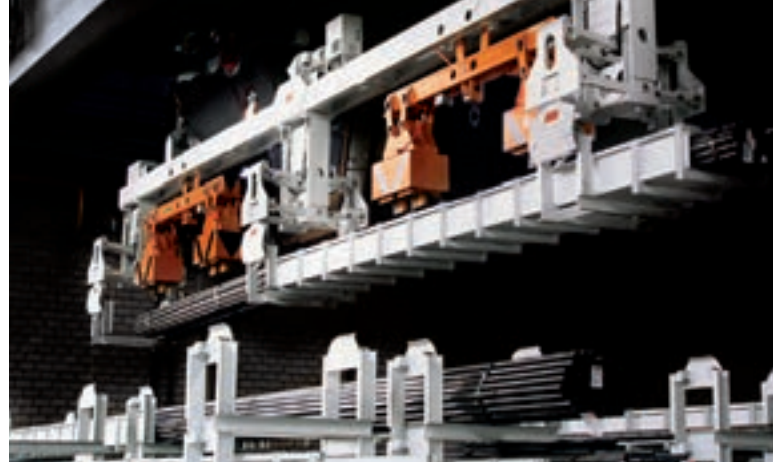
UNIBLOC F with combined spreader beam selectively for stacking cradle transport and bar removal.
