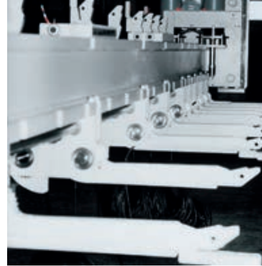
The KASTO loading traverse VarioPlus allows to pick up bars that are stored back to back.
