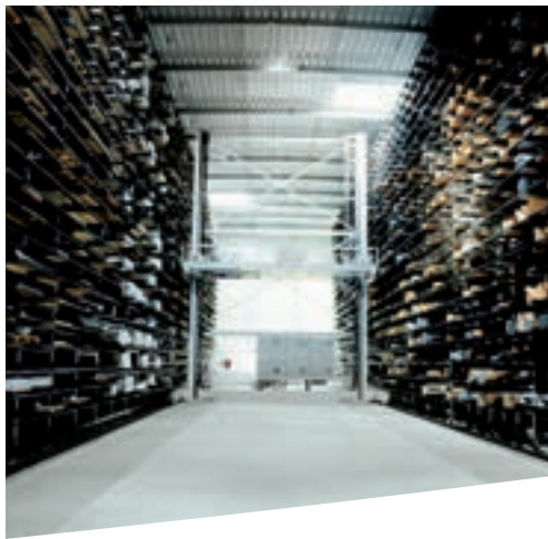
Honeycomb system with cassettes for long material and sheet metal pallets.
