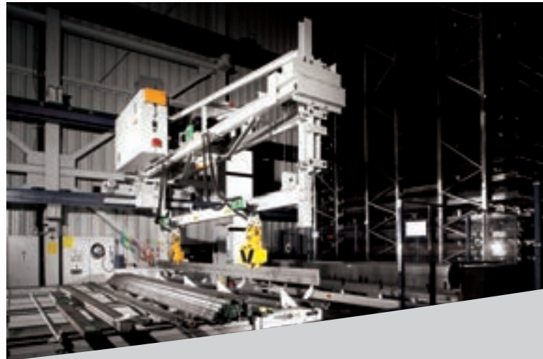
Order filling station with commissioning device with magnetic system and chain conveyor with tiltable commissioning trough.
