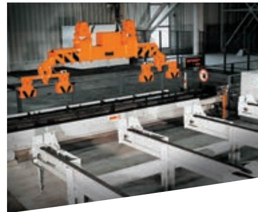
Magnet crane with pretensioned ropes for fast commissioning and loading onto an outfeed chain conveyor.
