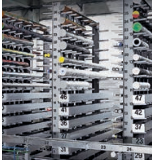
For individual bars and cassettes: KASTOcenter with a combined cassette and cantilever arm storage.
