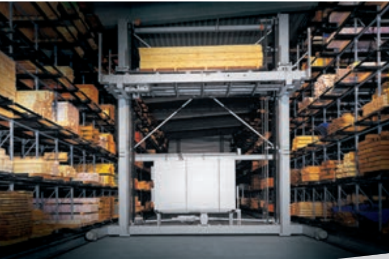
KASTOcenter: Combined storage-sawing-system with marking and palletizing device.
