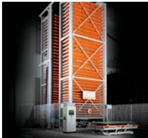
Storage system for sheet metal UNITOWER B for commissioning in service centers.
