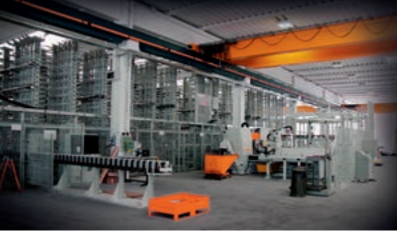
KASTOcenter: Combined storage-sawing-system with marking and palletizing device.
