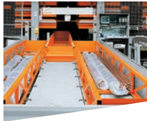
Commissioning stations with minimized cassette change times guarantee continu- ous production.
