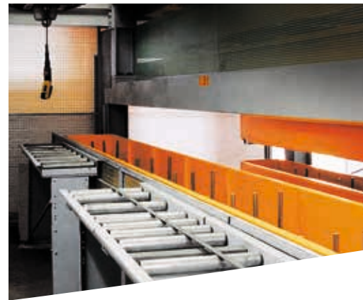
Connection of UNITOWER to a sawing machine by means of infeed roller conveyor.
