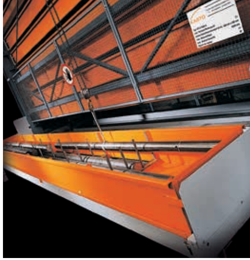
Lateral station cassette conveyor.
